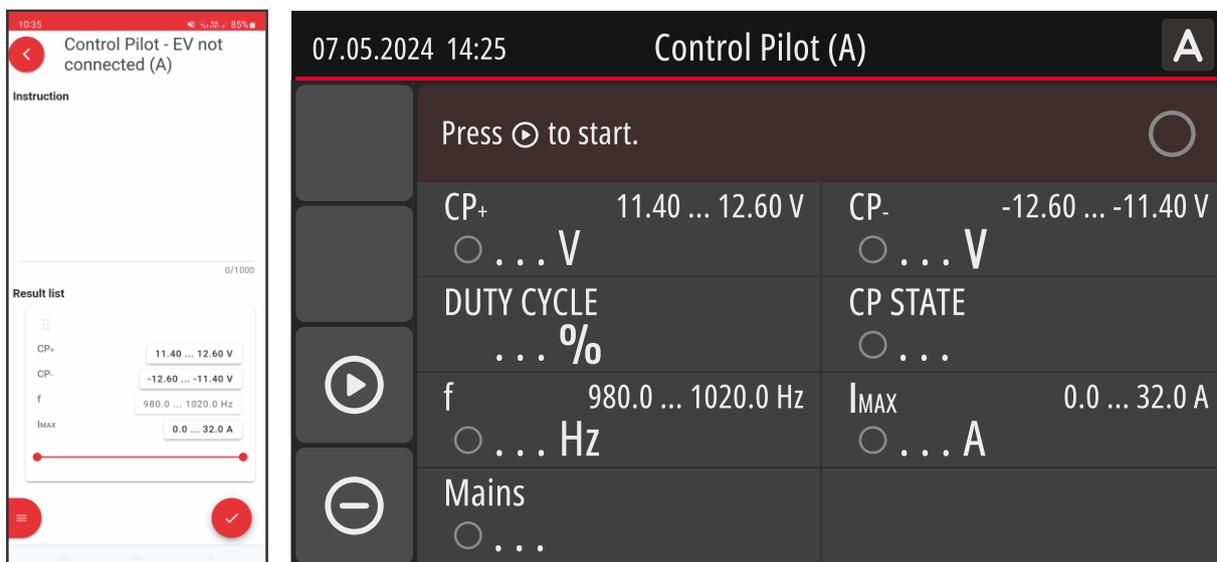
Figure 33: Control Pilot - EV not connected (A) "MiControl" application and measurement screen
