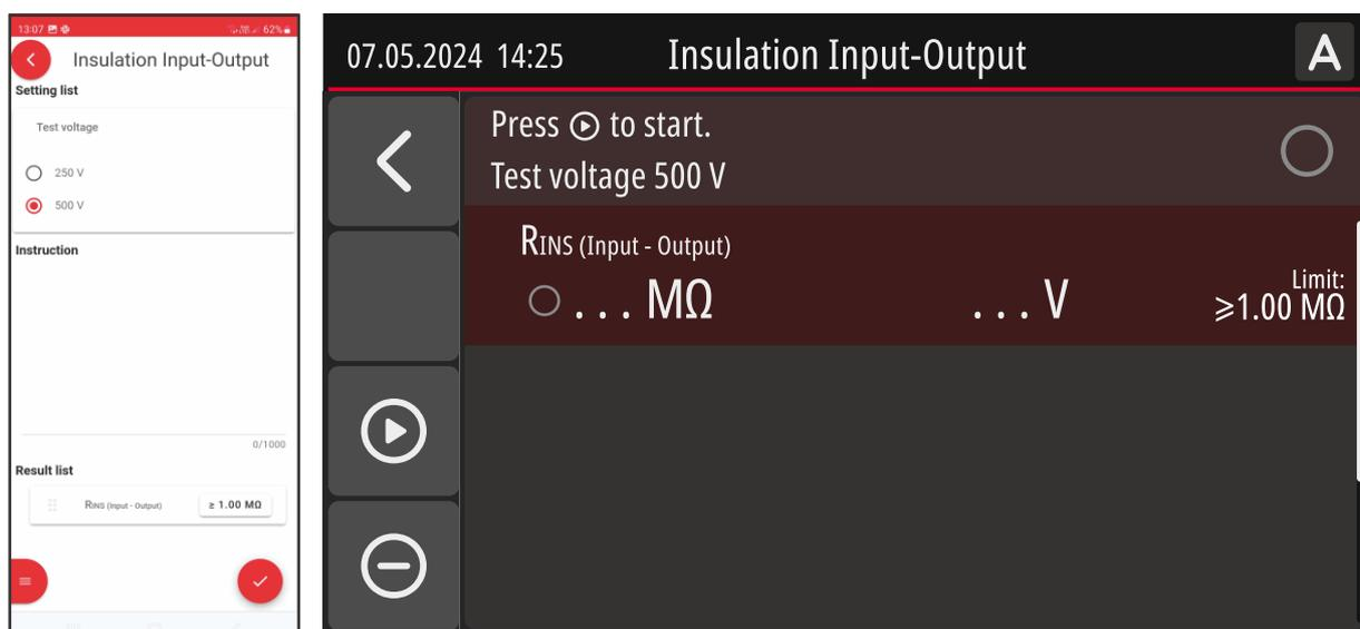
Figure 22:  $R_{INS}$  Input - Output "MiControl" application and measurement screen
