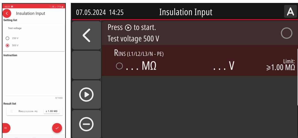
Figure 21:  $R_{INS}$  Input "MiControl" application and measurement screen
