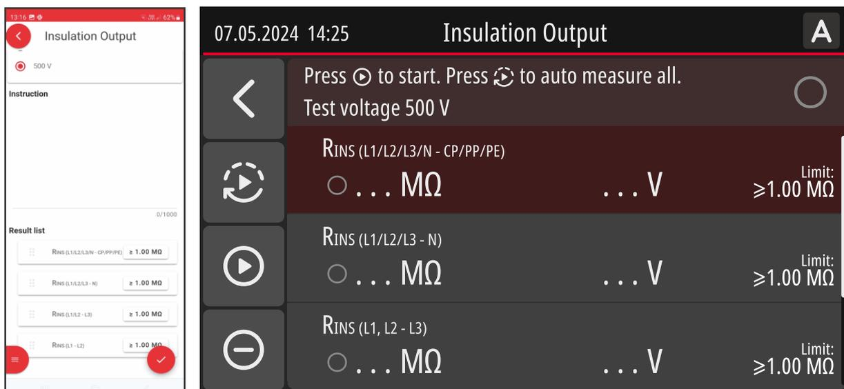
Figure 23:  $R_{INS}$  Output “MiControl” application and measurement screen
