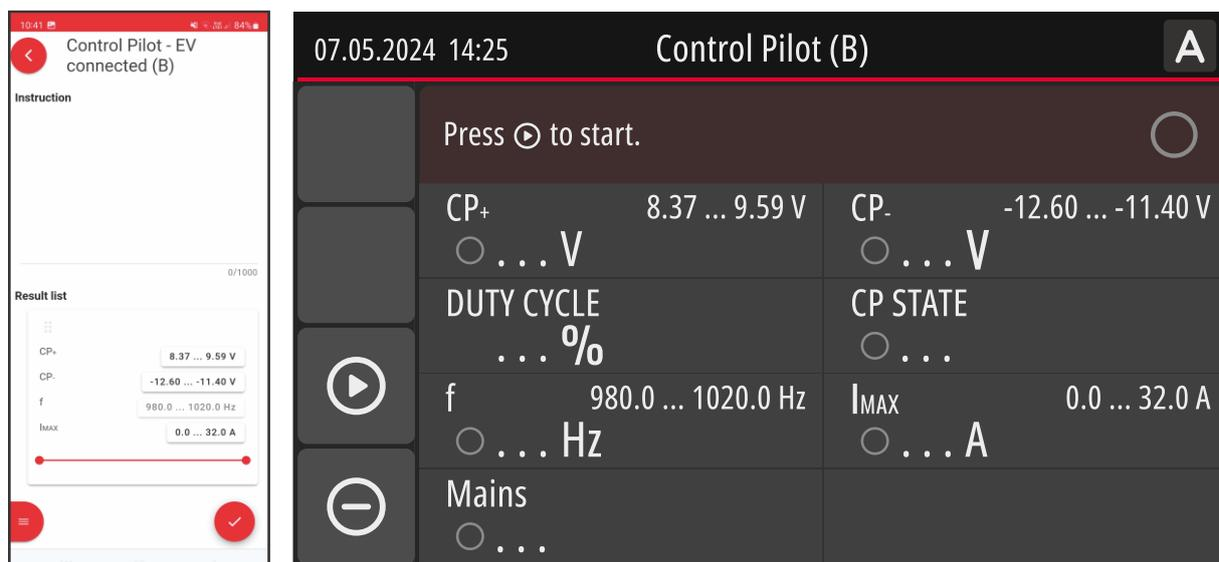
Figure 34: Control Pilot - EV connected (B) "MiControl" application and measurement screen
